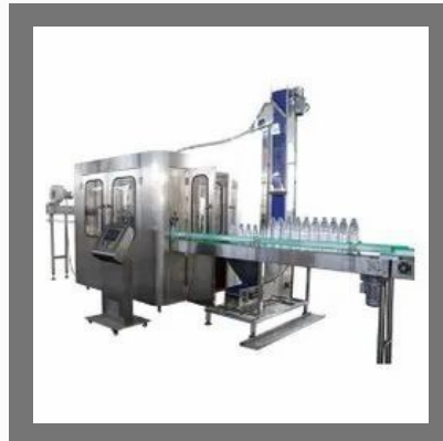
Automatic Mineral Water Bottling Plant
